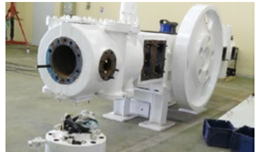
A volumetric compressor in the main workshop
